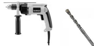
Hammer Drill w/ 1/4" Masonry Bit
